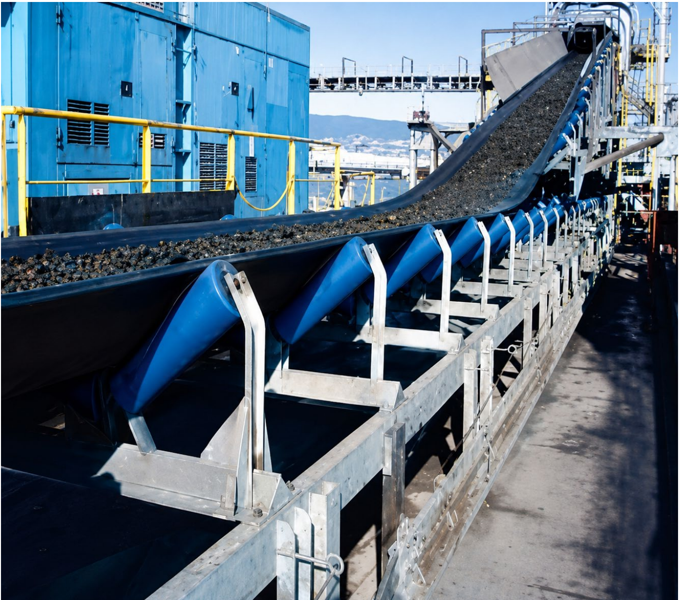
Typical polymer roller installation in a bulk-material belt conveyor.
